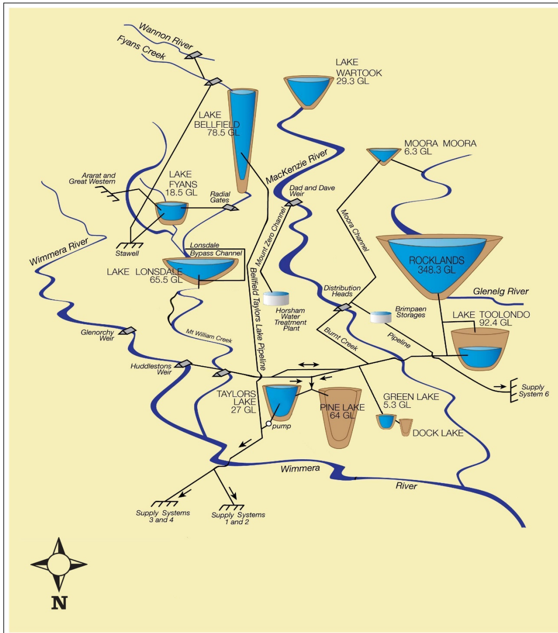
Figure 2.1: Schematic of the Wimmera-Mallee System Headworks (GWMW 2014), (not to scale, but shows relative elevation, depth, surface areas and connectedness of reservoirs)
