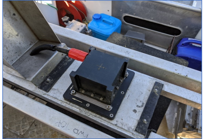
RTK GNSS observation taken on the IMU Z reference point
