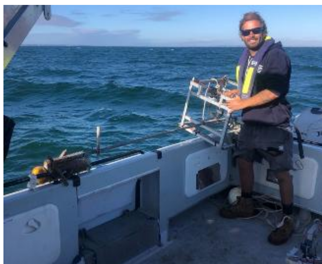
Figure 3. A Baited Remote Underwater Video prepared for deployment.
