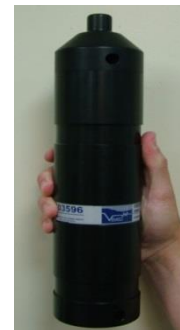
Acoustic receiver picks up the unique signal and records it along with the date and time
