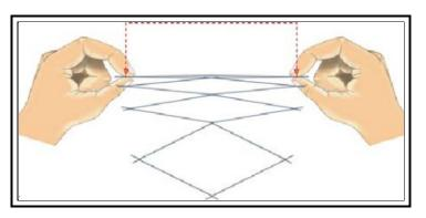
If there is any doubt concerning the measured mesh size, hang a 1 kilogram wight from knot 3 before the measurement is made.
